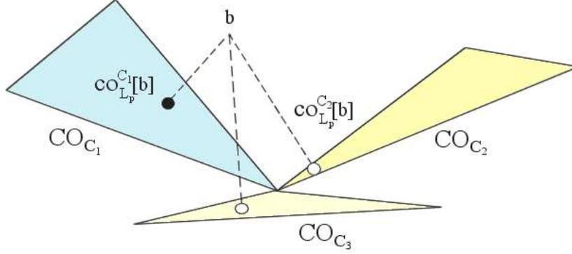
**Fig. 2.** To minimize the distance of a point from a simplicial complex, we need to find all the partial solutions (3) on all the maximal simplices in the complex (empty circles), to later compare these partial solutions to select a global optimum (black circle).
