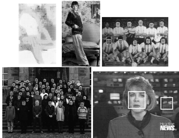
Figure 8. Top left: The darkness of the pixels of the left image are proportional to the number of reduced set vectors used to classify their associated patches of the middle image. Light grey corresponds to the use of a single reduced set vector, black to the use of all the vectors. Top middle: 153 \times 263 middle image contains 76108 patches and was detected in 2.58s. Top right: A 601 \times 444 image containing 518801 patches detected in 27.9s. Bottom Left: 1280 \times 1024 contains 2562592 patches and was detected in 80.1s. Bottom right: A 320 \times 240 image containing 147289 patches detected in 10.4s (Note the false positives).
