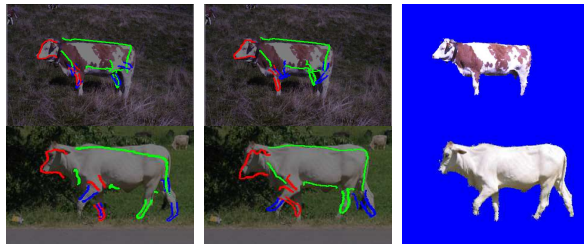
Fig. 14. The first column shows the initial estimate obtained for poses of parts of a cow in two images (see § V-B.1). The half-limbs tend to overlap since occlusion numbers are not used. Refined estimates of the poses obtained using the RGB distribution of foreground and background together with the LPS model are shown in the second column (see § V-B.2). The parts are shown overlaid on the image. The third column shows the segmentation obtained using the OBJCUT algorithm.
