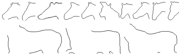
Fig. 9. The first and second row show the multiple exemplars of the head and the torso part respectively. The exemplars are obtained by establishing a correspondence between segmented images of cows and horses as shown in Fig. 8.
