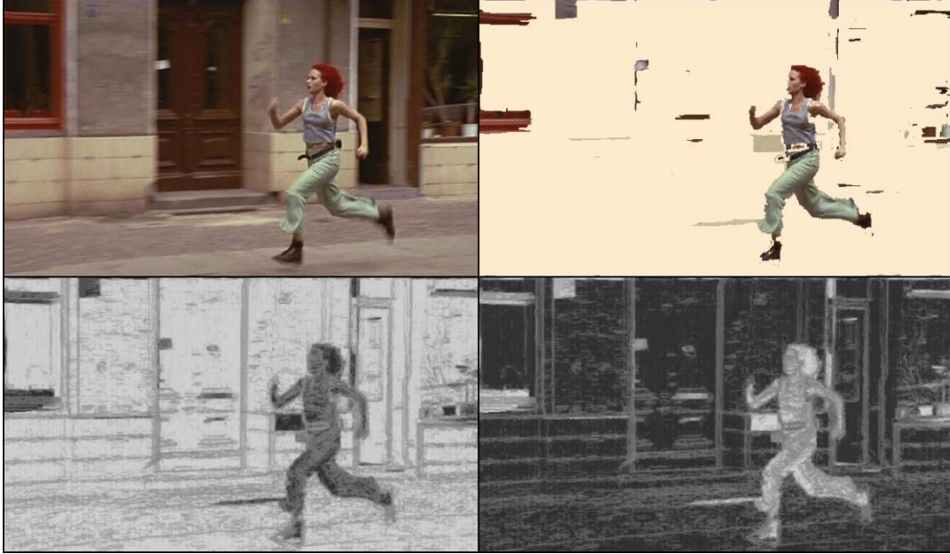
Fig. 7. Image segmentation with max-marginal probabilities. The first image is a frame of the movie Run Lola Run. The second shows the binary foreground-background segmentation where the aim was to segment out the human. The third and fourth images shows the confidence values obtained by our algorithm for assigning pixels to be foreground and background respectively. In the image, the max-marginal probability is represented in terms of decreasing intensity of the pixel. Our algorithm took 1.2 seconds for computing the max-marginal probabilities for each latent variable label assignment. The time taken to compute the MAP solution was 0.3 seconds.
