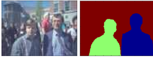
Fig. 5. The figure shows a keyframe of the ‘Dayton’ sequence, and the corresponding user specified segmentation. This segmentation was used to learn the patch dictionaries for the three segments namely background, human1 and human2.
