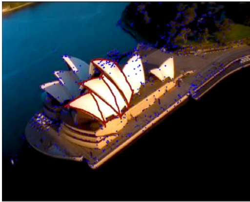
Figure 6: Generating NURBS surfaces from boundary curves in the absence of reconstructed object points.
