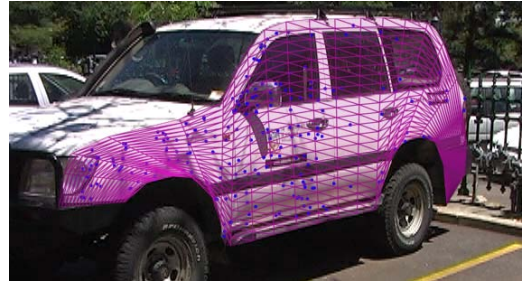
Figure 8: NURBS surface fitted to reconstructed object points.
