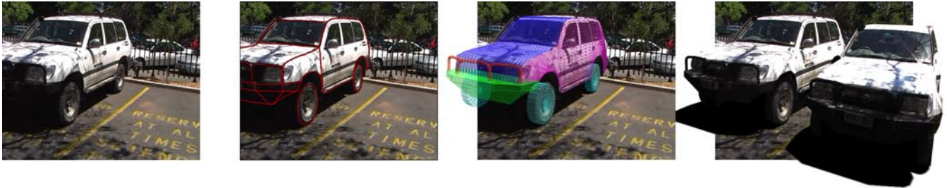
Figure 1: Left to right: a frame from the input video sequence, a partial tracing of the model, the final model overlaid on the video, and the result of rendering the final model back into the original sequence.
