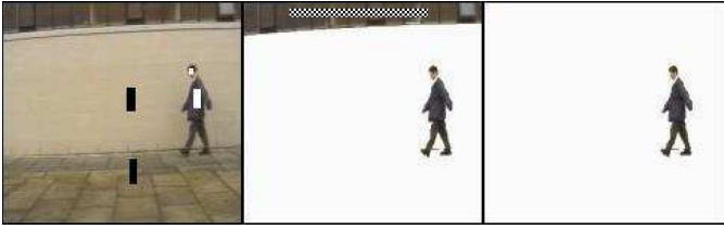
Fig. 6. Segmentation in Videos using user seeds. The first image shows one frame of the input video with user segmentation seeds (the black and white boxes). The image pixels contained in these boxes are used to learn histograms modelling foreground and background likelihoods. The second image shows the segmentation result obtained using these likelihoods with the method of [4]. The result contains a certain portion of the background wrongly marked as the foreground due to similarity in colour. This error in the segmentation can be removed by the user by specifying a hard constraint. This involves marking a set of pixel positions in the wrongly labelled region as background (shown as the checkered region in the second image). This constraint is used for all the frames of the video sequence. The third image is the final segmentation result.
