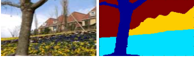
Figure 2. Segmented keyframe of the garden sequence. The left image shows the keyframe while the right image shows the corresponding segmentation provided by the user. The four different colours indicate pixels belonging to the four segments namely sky, house, garden and tree.
