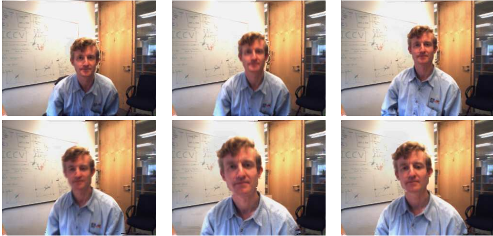
Fig. 32. Cyclopean image synthesis for long sequences. Some frames of a cyclopean video sequence synthesized by 4-state DP. The two input left and right sequences are not shown here.
