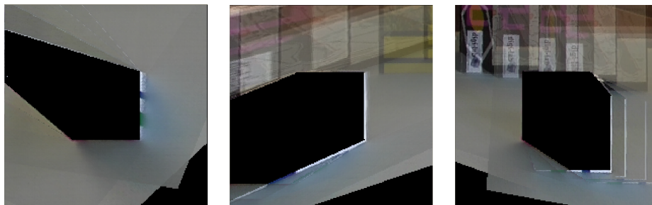
Fig. 4. The reprojection of the image set corresponding to 3 plane hypotheses with visibility masked areas shown in black. The leftmost representing the correct hypothesis
