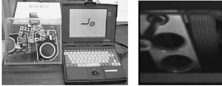
Figure 4. The PantoMouse planar robot ( left ). Its pose is just the 2D position of its end-effector ( right ).
